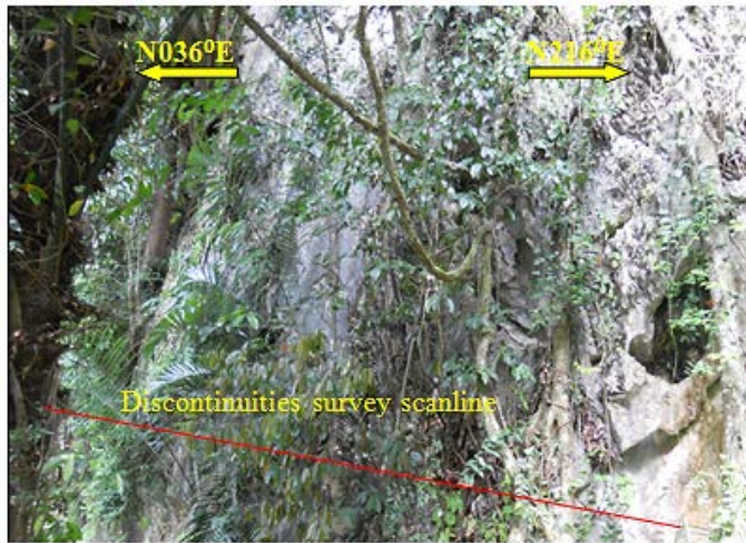
Figure 9: Discontinuity survey scanlines at the outcrop of slope GT for Gua Tempurung, Gopeng, Perak
