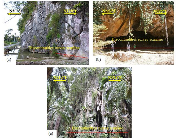
Figure 6: Discontinuity survey scanlines at the outcrop of (a) slope GK1, (b) GK2 and (c) GK3 for Gua Kandu, Gopeng, Perak
