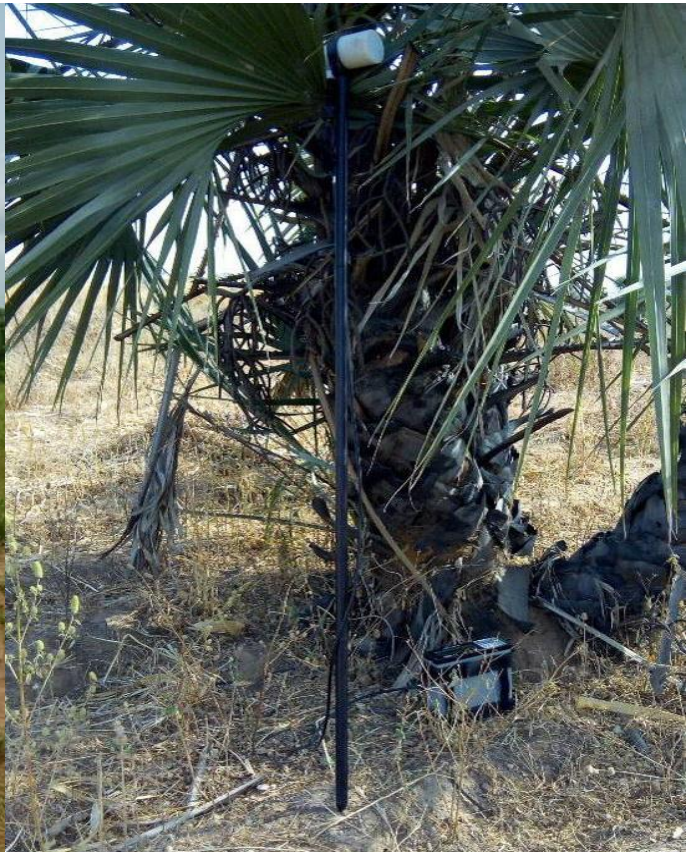
Plate 1: Magnetic Data acquisition (Rover) and Plate 2: Magnetic Data acquisition (Base)
