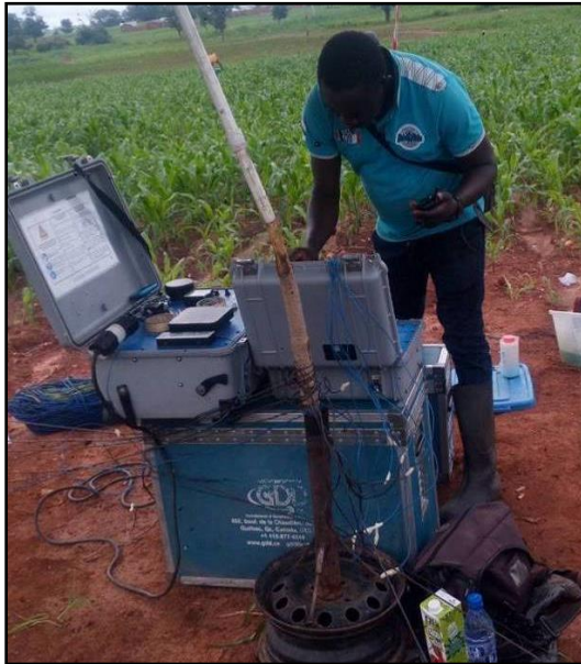
Plate 3: Data Acquisition with GDD IP System and Plate 4: Porous pot and connecting cables
