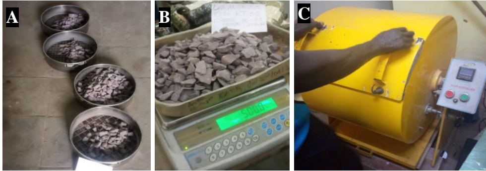
Figure 5: Conduct of the test. A: Sieve; B: Libra; C: Los Angeles camera.
