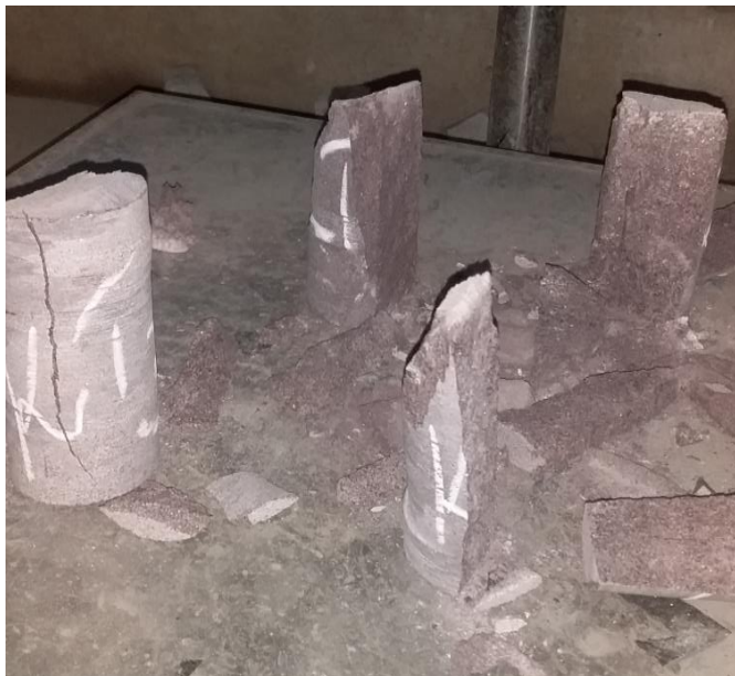
Figure 14: Specimen NZ01, NZ02, BB01 and BB02 after testing.
