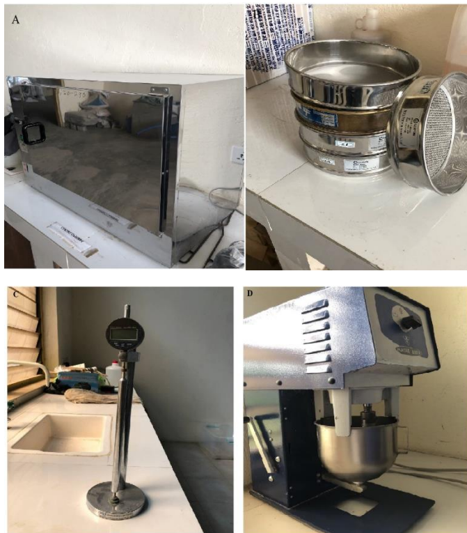
Figure 6: (A) Curing Cabinet; (B) Test Sieves; (C) Length comparator; (D) Concrete mixer
