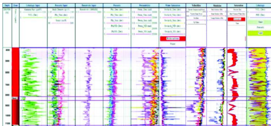
Figure 6: Basic log, Petrophysical and Geomechanical Properties of Well R08 showing two sand units.
