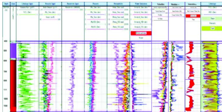
Figure 5: Basic log, Petrophysical and Geomechanical Properties of Well R07 showing two sand units
