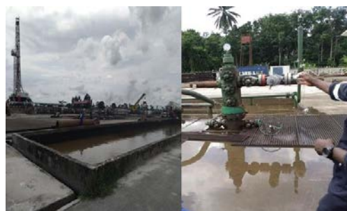
Figure 2: a. Shows sludge generated during drilling operations. b. Shows one of the well heads at the oil field.
