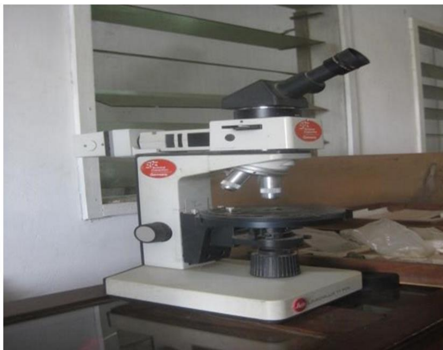
Figure 1: Petrographic microscope used to analyze the minerals present in the rocks.
