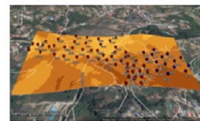
Figure 6: Cohesion distribution mapping by using Ordinary Kriging layered on Google Earth
